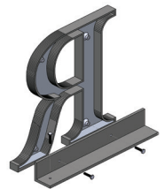
3D - Bottom Back Angle Bracket Mount Letters 4"-24", Minimum 3/8" thick. Letters over 12" may require tie-back (not supplied). Angle iron is 2" x 2" with a painted finish.
